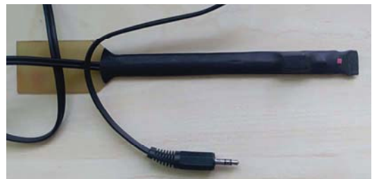
Fig. 4. Transverse magnetic field probe based on the A1324 sensor IC.
