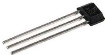
Fig. 2. A1326/24 low noise, linear Hall-effect sensor ICs with analog output, 3-pin ultramini SIP (1.5 mm x 4 mm x 3 mm).
