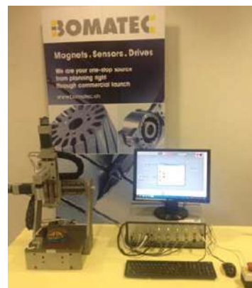
Figure 4. Bomatec AG utilizes the SENIS Magnetic Field Mapping System for quality control of permanent magnets.
