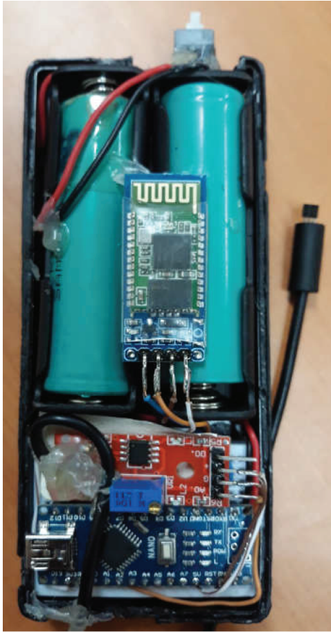
Figure 3. Typical set-up using the Arduino.
