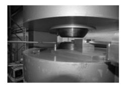
Fig. 31: Left: Hall probe inside a 2 T calibration magnet. The magnet has a gap of 38 mm and a field homogeneity  $0.6 \times 10^{-5}$  in the centre. Right: Measurement of the Hall voltage  $V_H$  for a magnetic field read by a NMR probe *B-NMR*
